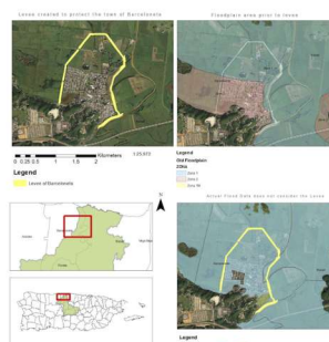
Figure 3: Floodplain area and levee constructed around the town of Barceloneta. Source: USGS
